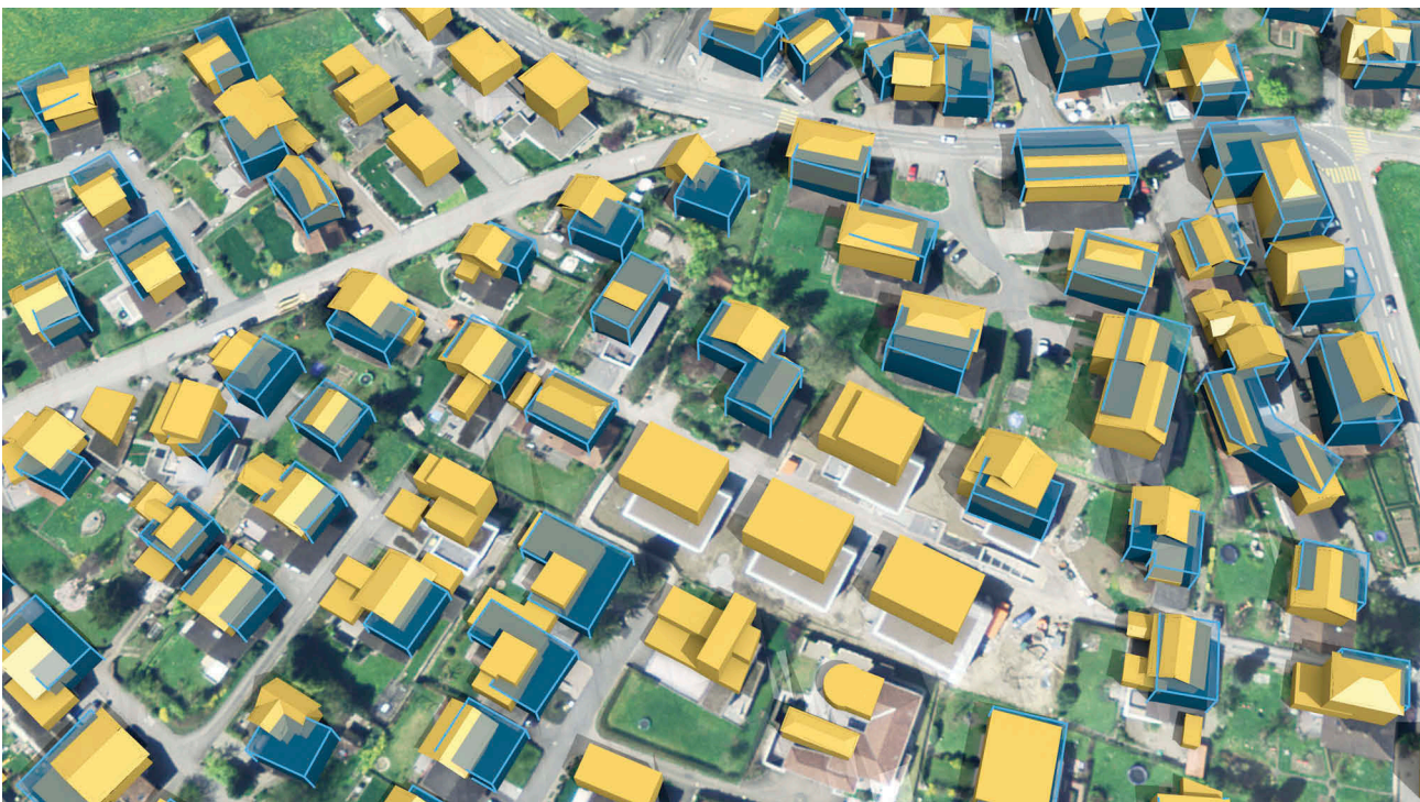
Figure 4. Two datasets of different LODs overlaid on an orthophoto (LOD1 – blue and LOD2 – yellow) of the same area but of different accuracy. The models are produced in separate campaigns, resulting in different positional accuracies and varying completeness. Data (c) Swiss Federal Office of Topography.
